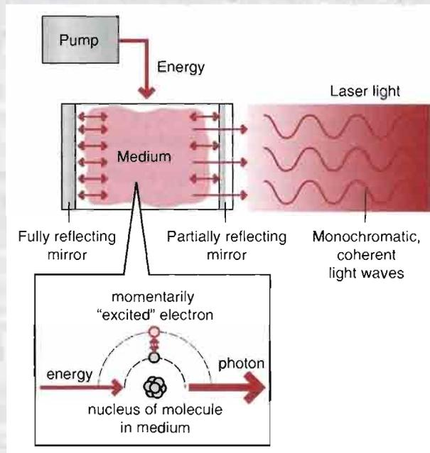
Laser production requires four essential components: (1) an active (amplifying) medium, (2) a mechanism for exciting the medium (a pump), (3) a reflective mirror, and (4) a partially reflective mirror that allows for some transmission of light and reflects the rest.
