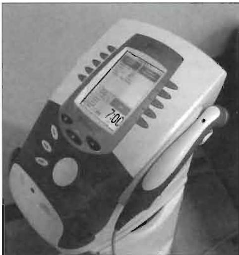
**Figure 8-8. Ultrasound—Electrical Stimulation Combo Unit.** These devices are electrical stimulators and ultrasound generators housed in the same unit. Electrical stimulation and ultrasound can be applied at the same time (see Ultrasound and Electrical Stimulation).
