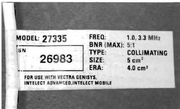
**Figure 8-1. FDA Labeling Requirements for Therapeutic Ultrasound.** The sound head pictured here is capable of producing an output frequency of 1 or 3.3 MHz and has an effective radiating area of 4.0 cm<sup>2</sup>. Note that the BNR is listed as 5:1 for both outputs. The "Max." indicates that this was the maximum BNR found in a sample of sound heads.
